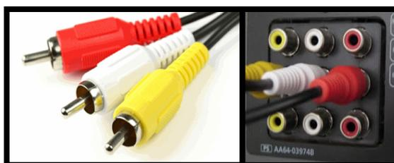
Composite cables and ports
