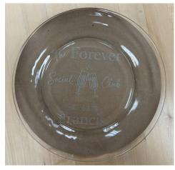
From Assistant Manager Michelle Mistalski: A patron came in looking to see if it was possible to engrave onto glass dishes. After creating a template on the laser cutter to the diameter of each dish, we were able to successfully center align, reflect, and laser etch the patron's design onto the back of each of the glass dishes. The patron was very happy with how they turned out and appreciated the efficiency in cutting out the template.
