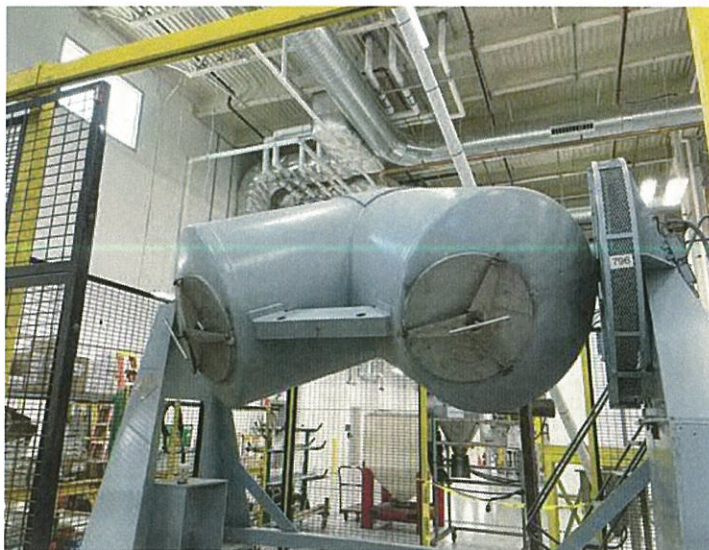
A cement mixer on steroids, ResinTech's "V blender" combines cation and anion resins at the ideal ratio to create thousands of cubic feet of mixed bed and other specialty medias. This is just one type of mixing utilized at ResinTech's new facility. ©ResinTech, Inc. All rights reserved.
