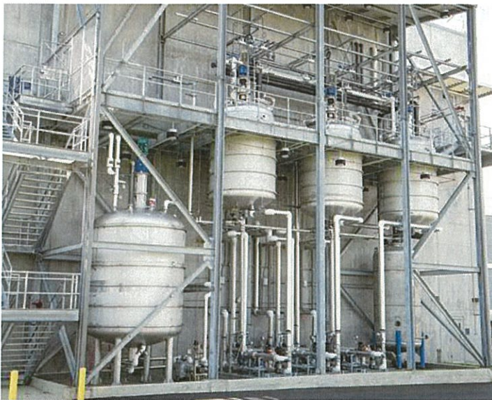
Jacketed reactor vessels control the extreme temperatures necessary to combine monomers into polymer, a precursor to functionalized ion exchange resin. ©ResinTech, Inc. All rights reserved.
