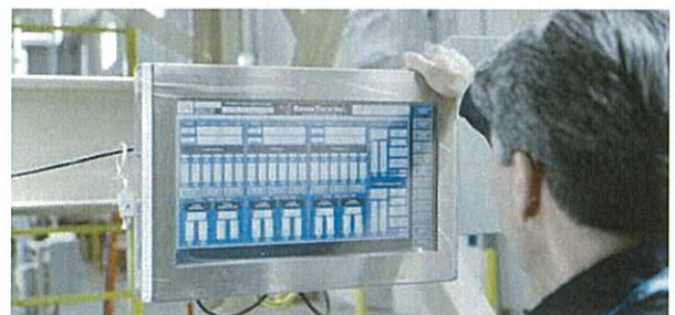
A dozen human machine interfaces (HMIs) help automate production while allowing engineers to monitor operations from anywhere on the 70,000 ft 2 production floor. ©ResinTech, Inc. All rights reserved.
